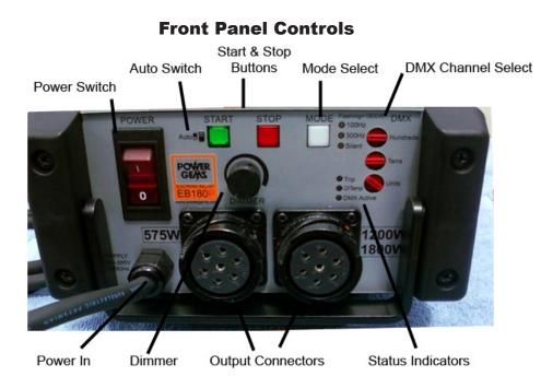
**POWER SWITCH:** The power switch is illuminated to indicate whether the switch is in the ON position, and that the ballast is connected to a power supply. The switch also acts as a circuit breaker to protect ballast in the event of a serious internal fault.
